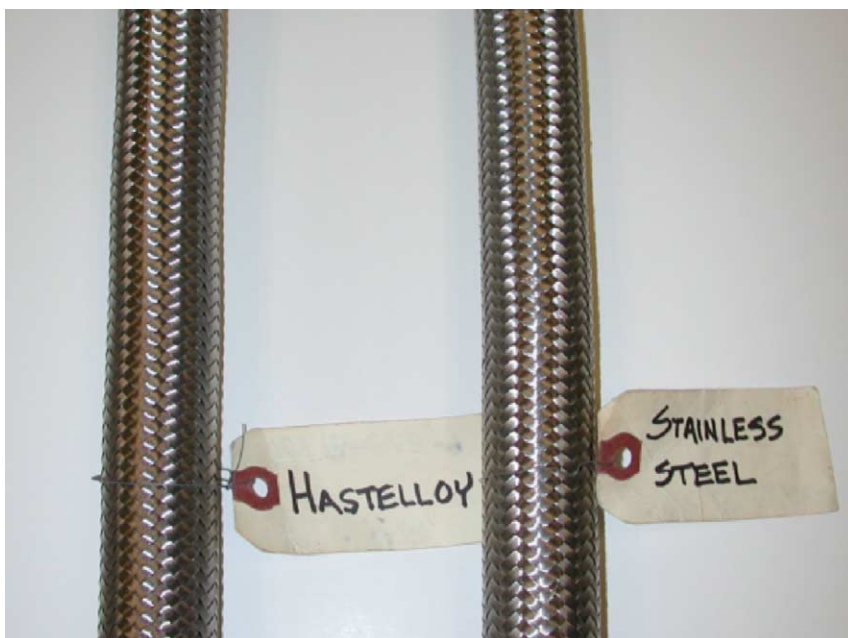
Fig. 1. Identical appearance of Hastelloy C-276 and 316L stainless-steel structural braiding.
